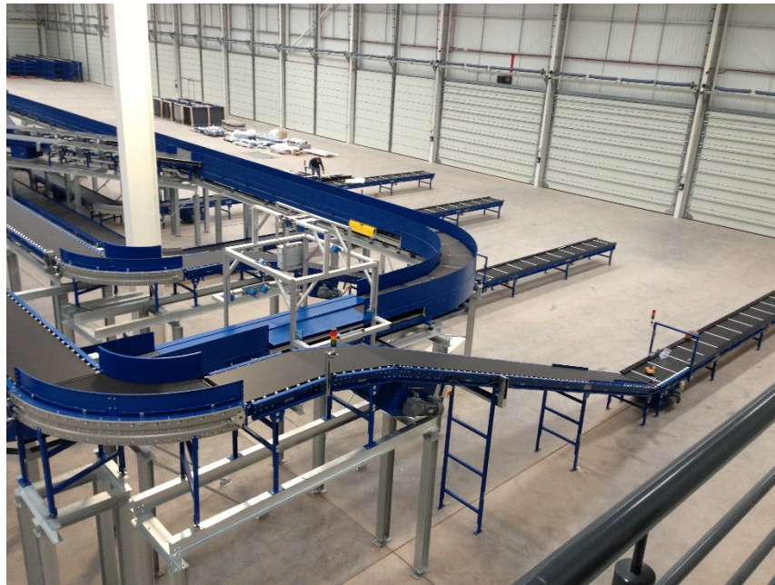
Heavy duty Belt Conveyor (Belt on Roller) for Parcel Sortation Hub running at 35m/min 70kg/metre capacity. In production since 2013.
