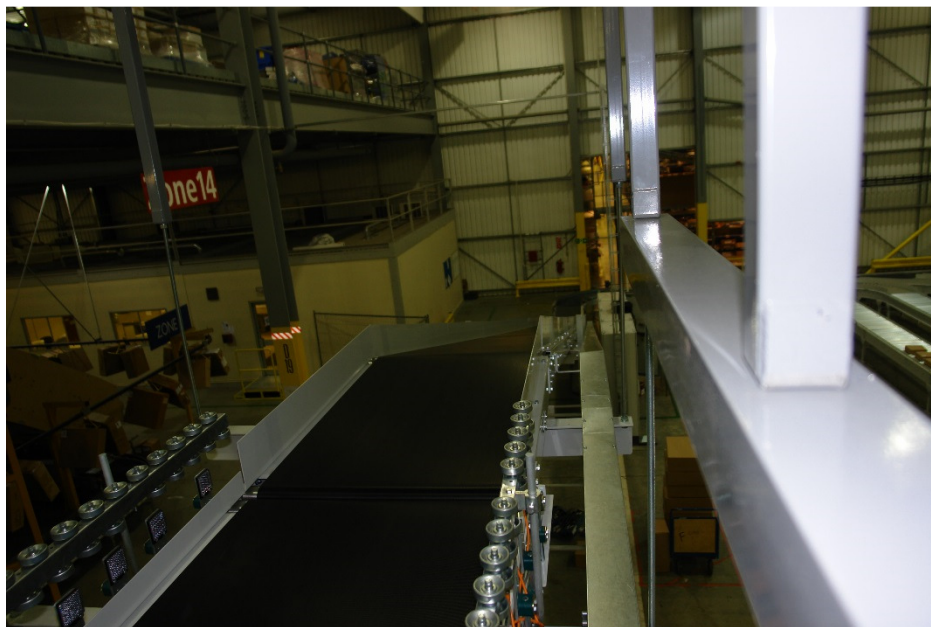
Heavy duty Belt Conveyor (Belt on Deck) for Parcel Sortation Hub running at 25m/min 50kg/metre capacity. In service 24 hours a day 7 days a week in production since 2006.
